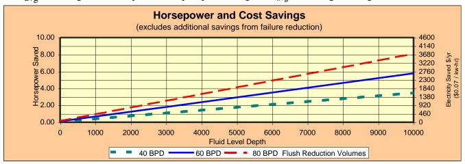
EXAMPLE: A well with a gate valve sidestream installation was tested and yielded a rate of 85 BPD (Barrels per Day) with an average wellhead pressure of 110 psi and a casing pressure of 80 psi. A SFR was installed and the flush was tested at 10 BPD. The pumping fluid level is around 5000 feet.
